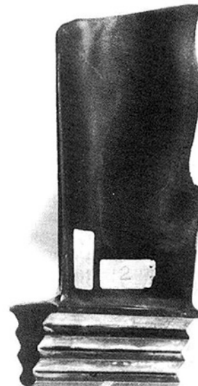
Fig. 1 Typical primary erosion characterized by thinning of the trailing edges
