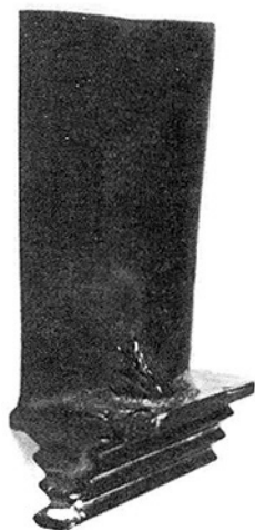
Fig. 2 Secondary erosion on an expander blade; most of the erosion is concentrated at the suction surface of the blade root aft of the midcord
